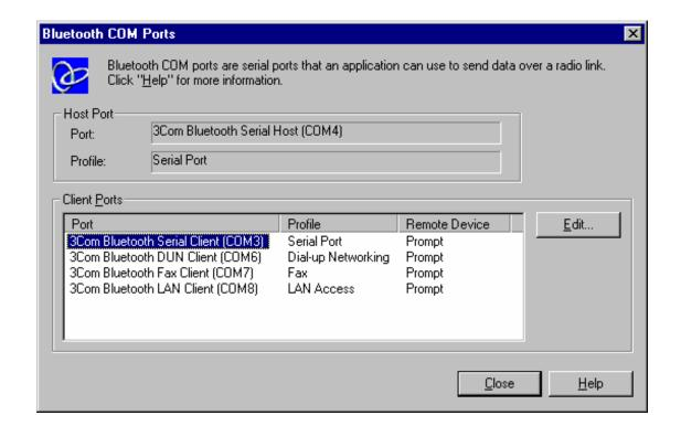
Install the printer driver, and assign it to the COM3 port which has been assigned 3Com Bluetooth Serial Client.
