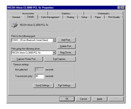
When printing is started from any application, this screen appears. Select the printer added to the Bluetooth device list as follows;
